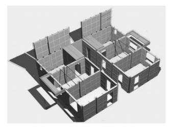
Fig. 1. Fibrous concrete wall structure system.
