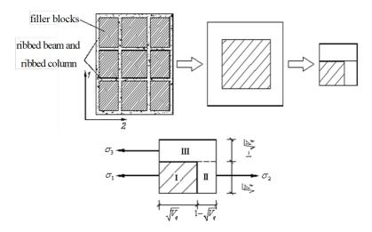
Fig. 6. Representative volume element of composite wall.
