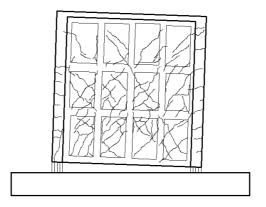
Fig. 3. Bending failure mode of the wall
