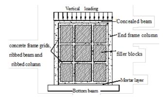
Fig. 2. Fibrous concrete wall.
