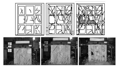
Fig. 4. Failure process of walls: from the left to the right elastic stage, elastic-plastic stage, failure stage.
